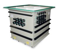
**KRASO® Pump Sump Type Q - Special** with 15 cm surrounding fixed-flange and water pressure tight surrounding KRASO® 4 Seal on the fixed-flange, reinforcing rips and concrete anchors and 35 water pressure tight KG pipe connections
