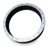
KRASO® Sealing Insert Type SD 150 - Special for KRASO® Casing Type FE or core drilling-d: 800 mm, non-corrosive stainless steel V2A, 150 mm seal against pressing water, external diameter media pipes: 1 x 679 mm
