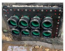
KRASO® Plastic Flange Plate Type KFP 150 Multiple 2x4 8 x 160 mm with welded KG 2000 spigot for the connection of a hose connection (10 cm protrusion length) MPA-tested up to 3 bar, plate made of 60 mm thick, highstrength special plastic, with EPDM flat seal, fixing and sealing
