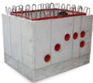
KRASO® Pump Sump - concrete - Special internal dimensions approx. 100 x 70 x 80 cm, made of waterproof concrete, with 20 cm thick, steel fibre reinforced wall and base plate (20 kg per cbm). Rebar connection approx. 8/15 two-rowed, surrounding water pressure tight, MPA-tested construction joint tape KRASOflex® Duo-Fix 150 „plus“, 4 lifting lugs M20, connections: 6 x DN 125, total weight: approx. 2.4 t
