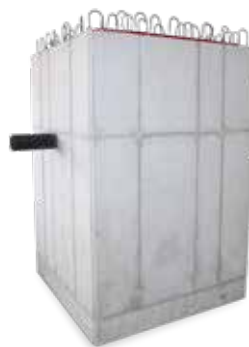
KRASO® Pump Sump - concrete - Special internal dimensions approx. 104 x 104 x 192 cm, made of waterproof concrete, with 20 cm thick, reinforced wall and base plate (20 kg per cbm), rebar connection approx. 8/15 two-rowed, water pressure tight surrounding, MPA-tested construction joint tape KRASOflex® Duo-Fix 150 „plus“, incl. PE pipe DN 124 with water pressure tight surrounding KRASO® 4 Seal with protrusion on both sides approx. 15 cm, 4 lifting lugs Rd20, total weight: approx. 5.94 t
