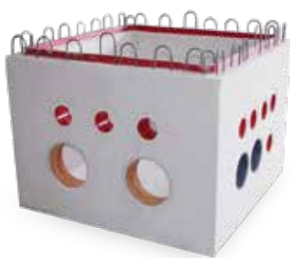
KRASO® Pump Sump - concrete - Special internal dimensions approx. 100 x 100 x 80 cm, made of waterproof concrete, with 12 cm thick, reinforced walls in one piece cast, rebar connection approx. 8/15 two-rowed, surrounding water pressure tight, MPA-tested construction joint tape KRASOflex® Duo-Fix 150 „plus“, 4 lifting lugs M20, connections: 8 x DN 110, 2 x DN 250, 2 x ID/FE 200, total weight: approx. 1.5 t
