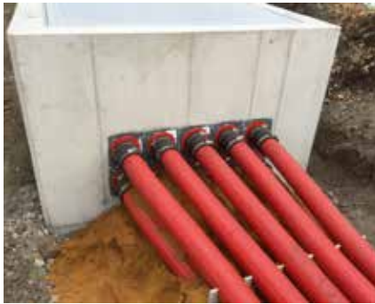
KRASO® Cable Duct - Special internal dimensions approx. 140 x 140 x 110 cm, incl. angle frame installation, made of waterproof concrete, with 20 cm thick, reinforced wall and base plates ( 20 kg/ per cbm ), without rebar connection/joint tape, 10 KRASO® Cable Penetrations KDS 150 on one side, according to drawing, 4 lifting lugs Rd20, weight/piece.: approx. 5 t
